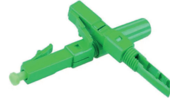
Mechanical connector SC Mod. FAB-FMC-LC30X20 • Application: Drop 3x2mm • RL: \geq 50 dB for UPC | \geq 55 dB for APC
