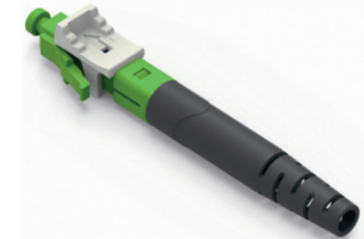
Mechanical connector SC Mod. FAB-FTD9201 • Application: 2mm, 3mm, 0,9mm & 3.0*2.0mm & Drop 2.0*1.6mm • RL: \geq 50 dB for UPC | \geq 55 dB for APC
