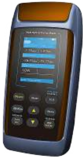
LP-3PX XG-PON Optical power meter
