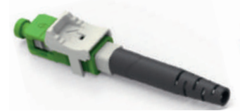
Mechanical connector SC Mod. FAB-FTD925U-L • Application: 2mm, 3mm, 0,9mm & 3.0*2.0mm & Drop 2.0*1.6mm • RL: \geq 50 dB for UPC | \geq 55 dB for APC
